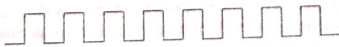
Fig. 3.27 Periodic clock waveform as seen on an oscilloscope displaying voltages versus time.
